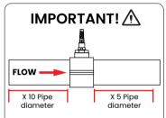
A minimum of 10x pipe diameter before (upstream of) the sensor and at least 5x pipe diameter after sensor of straight pipe section must be fitted with no bends, reductions, enlargements, restrictions or valves to ensure accurate measurement.
