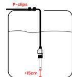
6 For open bodies of water, LX suggests purchasing the optional mounting bracket, available from incyt.io. Install using the diagram on the right as a guide, ensuring the sensor is located more than 15cm away from the ground, and is free from any obstructions such as rocks or debris.
