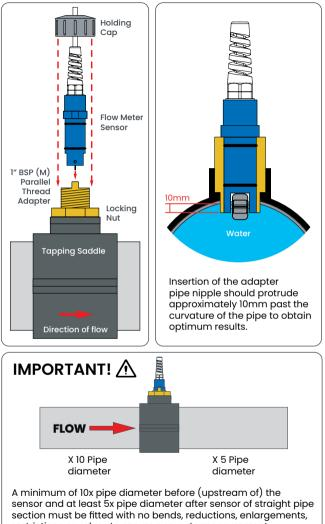
restrictions or valves to ensure accurate measurement.
