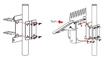
Attach the Solar Kit to the mounting bracket and secure with the supplied washers and wingnuts as above on the right. Orient the solar panel to maximise sun exposure throughout the day.
