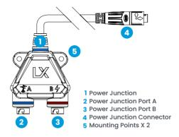
The Power Junction powers a Blue Node using an external power source (7-30V DC, 15W minimum). Compatible power sources include the USB-C to 6-pin Power Cable (BSUBPD15/BSUBPD60) and Solar Kit (LX-SK25).
