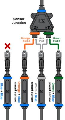
smart sensor cannot be used with the Sensor Junction
