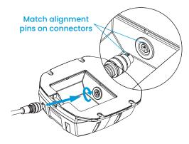
6 Connect the power cable to a suitable power source as in the example below. Detailed instructions are provided on the power cable packaging.
