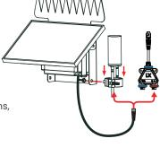
IMPORTANT! Base Station Antennas must point towards the ground!
